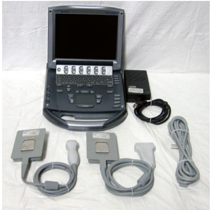
Fig. 1.3 A portable modern ultrasound scanner for intraoperative use (SonoSite M-turbo; SonoSite Inc, Bothell, WA, USA)
