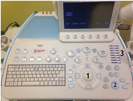
Fig. 3.1 Console of a commercial ultrasound system. A large number of commands can be seen, which are usually arranged differently among various vendors. However, three main commands are usually very similar regardless the brand. 1 trackball surrounded by four buttons, 2 freeze button, 3 time gain control setting
