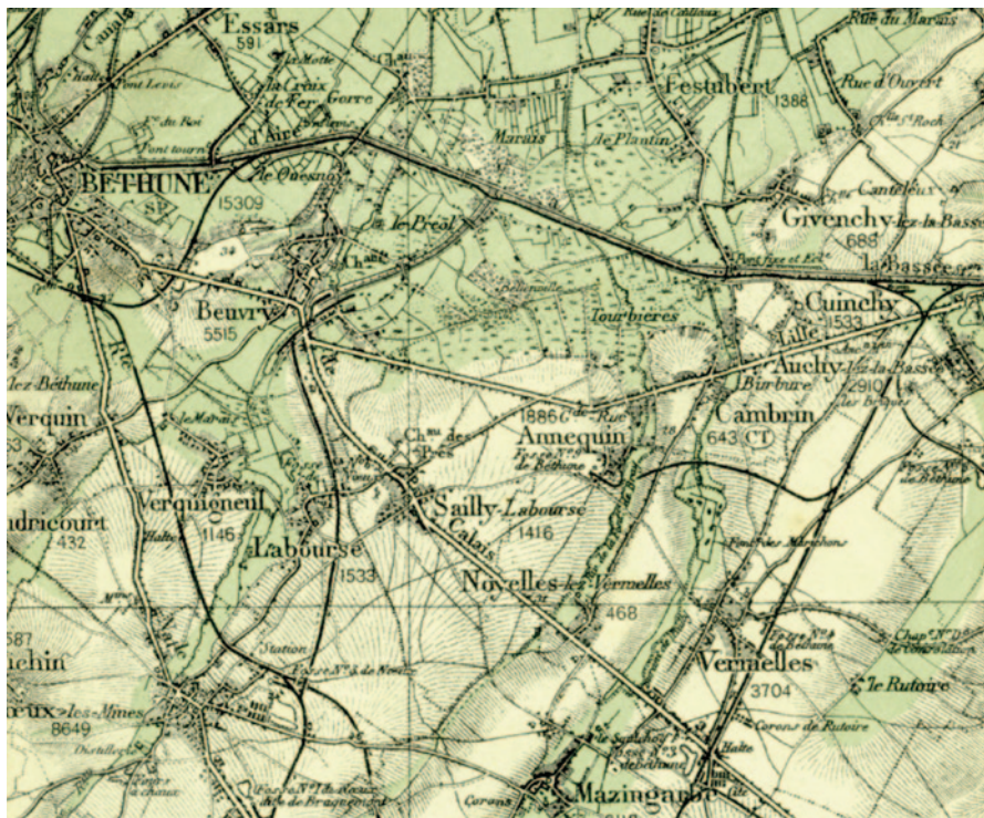
Fig. 15 During the early years of the war basic “Leerkarten” had no coloured areas. Later, valleys began to be overprinted in green. The extract shown is at a scale of 1:80,000
