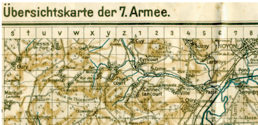
Fig. 10 The 7th Army was able to take a monochrome French map and turn it into a tri-color print (1:100,000), which was much easier to read. Mountainous terrain was shaded in brown , although there were no elevation annotations. Grid lines, each 1 km apart, made it possible to identify specific areas for reporting purposes
