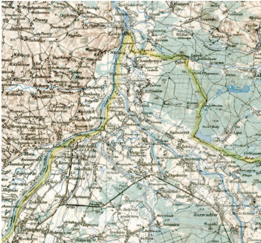
Fig. 22 Extract from a sheet of the Austrian General Survey Map 1:200,000 showing a well-designed four-color image (junction of the San and Weichsel Rivers near the Russo-Polish border). A hand-drawn yellow line indicates the border itself. Although the overall appearance of the map is appealing, the cartographic quality of areas outside Austrian territory was definitely poor, a fact which led to many military difficulties, especially in the southern Balkans
