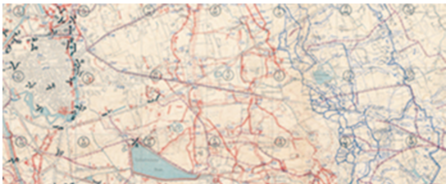
Fig. 14 The 4th Army at Ypres could draw upon existing Belgian maps. The extract shows a trench map on a scale of 1:20,000. The 1 km grid lines indicate the use of a coordinate system designed specifically for army use. Upon examination of the index map, however, it is evident that the scale of 1:20,000 was still much too small for accurate operation planning at the front
