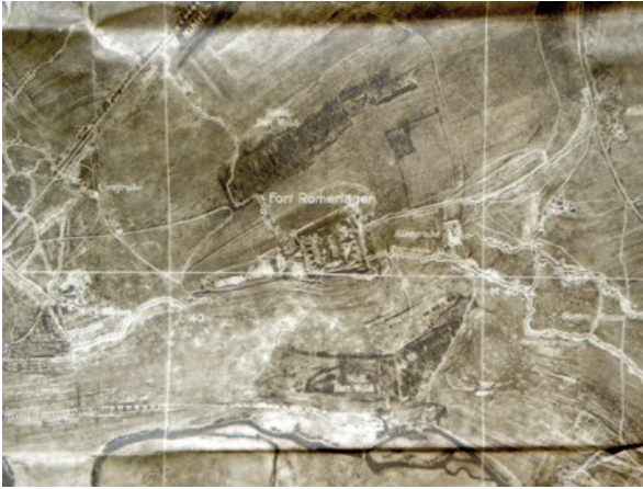
Fig. 16 Aerial maps ( Luftbildkarten ) (see Table 1, no. 7) were made with the help of a complex series of different photos, enhanced by toponyms and a map grid. Above, a sector of such a sheet. Such a map could give the troops a good impression of the actual situation, but they had to learn how to “read” an aerial map. These maps provided almost no information on the surface contours. Because everything seemed flat, the officers in command wanted both: The normal contour sheet as well as an aerial map. The British forces created similar maps. (Chasseaud 2013, p. 207)
