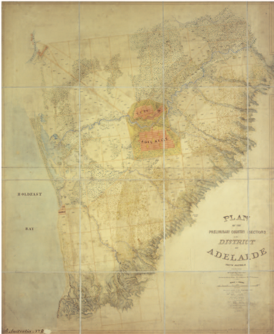
Fig. 16 Plan of the Preliminary Country Sections in the District of Adelaide as surveyed by Wm Light Esqr and Assistant Surveyors. The first points for the Trigonometrical Survey were fixed by Messrs. Light, Ormsby, Finnis and Cannan. In the town Mr. Jacob. In the field Messrs. Pullen, Lindsay, Hardy, Simmonds and Mr Winter. Drawn by Henry Nixon, late Lieutenant 96th Regiment. (Courtesy of the British National Archives, CO 700/SOUTH AUSTRALIA2Pt1(4))
