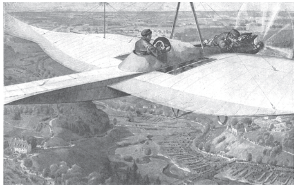
Fig. 3 A Type A plane on a reconnaissance flight in 1914. The pilot sits in the rear and the observer in front. The observer uses binoculars but has no camera. The map board can be seen on his left. ( Illustrierte Geschichte des Weltkrieges , no 11, p. 218)
