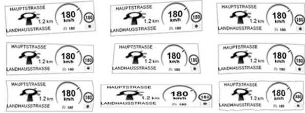
Fig. 3 Distortions caused by assembly tolerances of the HUD housing (illustration adapted from Jordan 2014, distortion types according to Eichhorn and Zink 2012 and Neumann 2012)
