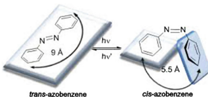
Fig. 4 Photoisomerization process of azobenzene [5]
