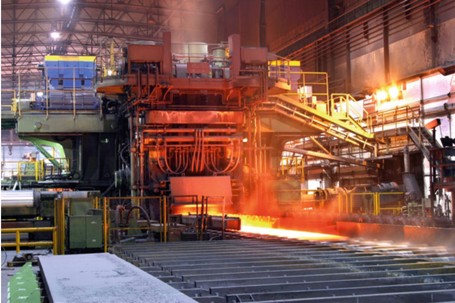
Fig. 7.15 Steel slab in the hot rolling mill—with permission from Salzgitter Flachstahl GmbH
