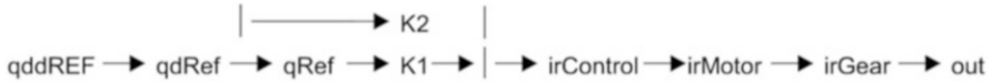
Fig. 5.9 Composition diagram of one axis of the robot manipulator in Fig. 5.8 (For details see text)
