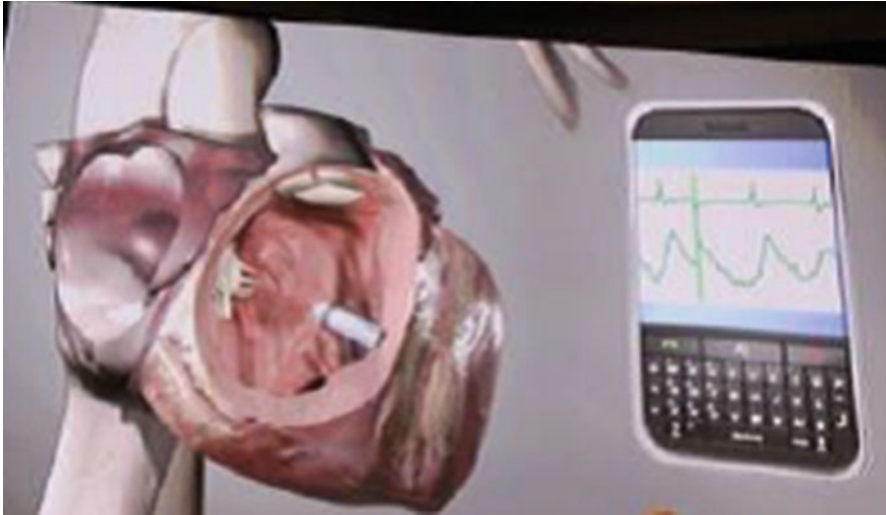
Fig. 3.6 Wireless pacemaker implanted directly into the heart chamber and extracorporeal monitoring by a nearby smartphone ( http15 2015)
