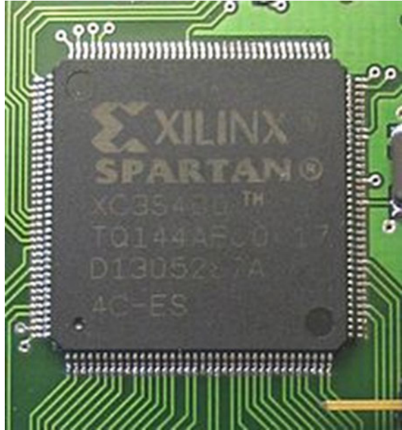
Fig. 5.5 Xilinx FPGA Spartan XC3S400 ( http://www.xilinx.com/products/fpga/xc3s400/ )
