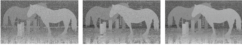
Fig. 2. Combination of two disparity maps in different directions. The left is the horizontal disparity map. The middle is vertical disparity map. The right is the result.
