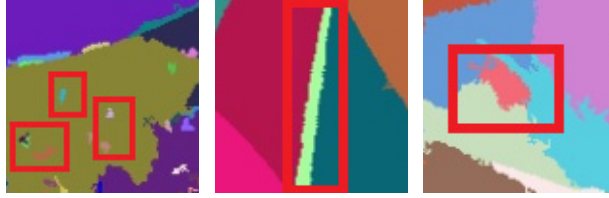
Fig. 3. Threshold in region merging. Regions in red rectangle need to be combined. The left is small region in a huge region. The middle is thin and long region between two regions. The right is small region surrounded by several regions.
