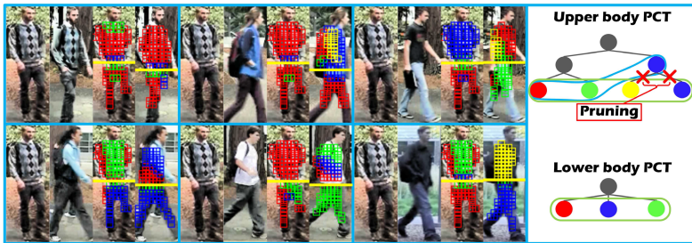
Fig. 3. Different colors of leaf nodes represent different clusters. Specially, upper body patches are clustered to 3 or 4 clusters under our pruning condition.
