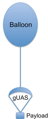
Fig. 1. A conceptual sketch. A small weather balloon carries the payload to a desired altitude. Once released from the balloon, the gliding UAS (gUAS) brings the payload back to the launch point. The payload takes data during both ascent and descent.
