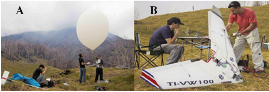
Fig. 6. (A) SO 2 -sonde package ready to be lifted as part of a tethered balloon aerostat on the slopes of Turrialba Volcano. Note the severe vegetation damage due to SO 2 and CO 2 poisoning, in the background. (B) UCR crew pre-flights the Vector Wing 100 UAV on Turrialba (Photo: J. Linick, JPL).
