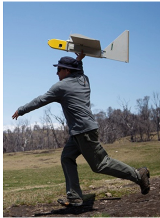
Fig. 4. NASA Dragon Eye, originally built in 2001 by Aerovironment Inc. This small (0.9 m length, 1.1 m wingspan, 2.7 kg weight) is a rugged and versatile platform for deployment of small sensors ( \leq 500 g) into volcanic plumes. It cruises at 65 km/h over a 5–10 km range and flies completely autonomously with automatic ascents and landings. The current NASA ARC Dragon Eye fleet consists of 75 aircraft plus spares, operated by the NASA Airborne Science Program (Photograph: Justin Linick, JPL).
