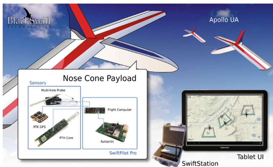
Fig. 5. Illustration of prospective Apollo multi-UAV-based sensorweb showing an intuitive user interface. Currently under development within the NASA SBIR Program (courtesy of J. Elston, BlackSwift Technologies).
