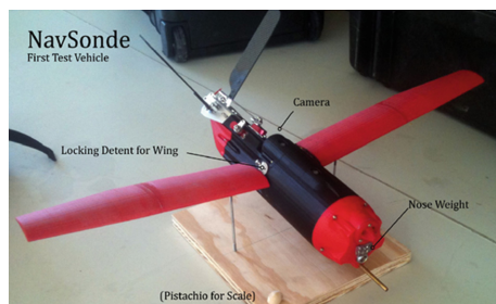
Fig. 3. The steerable NavSonde vehicle by Latitude Engineering, Tucson, AZ. A glidesonde under development within the NASA SBIR Program, it can carry a volcanic ash sampler, camera, or electrochemical gas sensors. It is recoverable, and can be tube-dropped from a standoff vantage point to penetrate volcanic ash plumes—minimum 10:1 glide ratio (Courtesy of Latitude).
