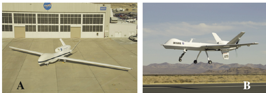
Fig. 1. (A, left) NASA Global Hawk, for use in high-altitude, long-duration Earth science missions, 13.5 m in length, with a wingspan of 36 m, payloads up to 900 kg and at altitudes of up to 20 km. Its range is greater than 18,500 km and its endurance is greater than 31 h. Dropsondes for nadir deployment into volcanic clouds would be a possibility from Global Hawk—neutral buoyancy heights of most explosive eruption plumes are below the operational ceiling of this aircraft, thus dropsondes or glidesondes could be deployed from this platform, or from Ikhana (B, right) NASA Ikhana, named after the Native American Choctaw word for intelligent, conscious or aware . NASA uses this airborne platform for a variety of long-duration Earth science missions, and to demonstrate and validate electronic sensor technologies. The enlarged fuselage nose accommodates various payloads, including imaging systems, LIDARs and radars. The aircraft is 11 m in length, with a wingspan of 20 m. (Photograph: NASA).
