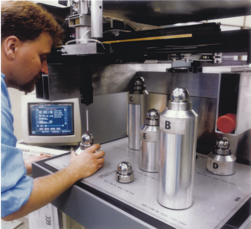
Fig. 5.9 The calibration of a CMM, utilising a ‘3-D ball-plate’—where the major benefit being here to have differing sphere positions/heights—supplied on a purpose-built fixture, when calibrating the equipment (courtesy of Renishaw plc)
