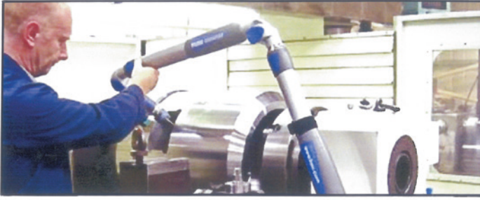
Inspecting critical dimensional features of an accurate & precise turned component employing an 'articulated arm'. [Courtesy of FARO Technologies Inc]
