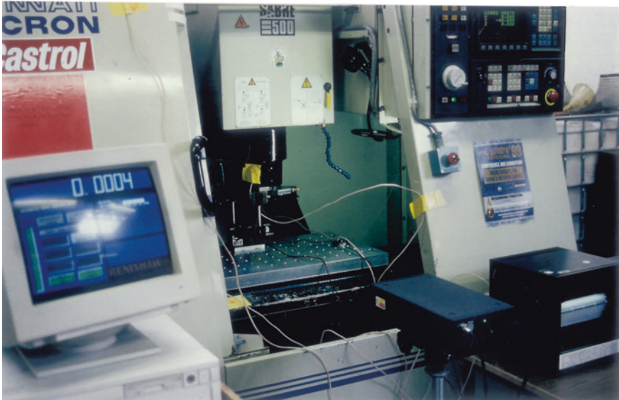
Fig. 5.18 Calibration of a vertical machining centre, prior to high-speed machining trials on a stereometric artefact [after: Smith et al. (2001)]
