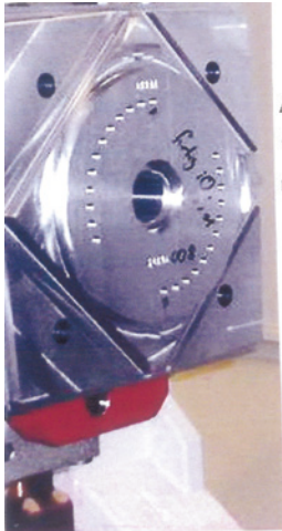
A typical 'Machinable artefact': NAS 979 'Composite Cutting Test', that has been machined on a horizontal Machining Centre.
