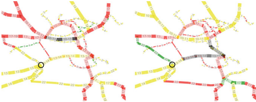
Fig. 9.11 Volume over capacity changes due to disruption scenarios—on the southbound Blue lines 10 and 11 ( left ) and the southbound Red lines 13 and 14 ( right ). The disrupted sections are shown in black . Sections with more than 5 % relative increase in volume-over-capacity ratio are depicted in red ; yellow corresponds to no significant change, and sections with a relative decrease of more than 5 % are shown in green . The link labels correspond to the line numbers, and the Liljeholmen transfer hub is marked with a circle
