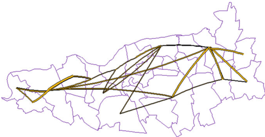
Fig. 9.3 The segmentation of a territory in zones ( in purple ) and the representation of the OD flows by desire lines ( in yellow )
