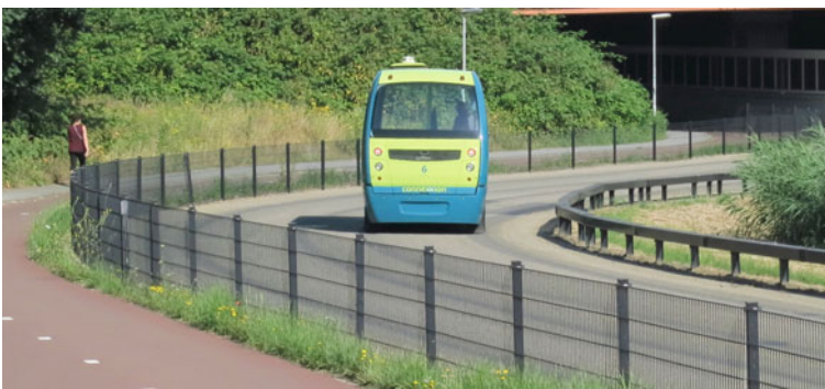
Fig. 2.32 Automated minibus in regular service on special busway in Rotterdam (Kottenhoff, June 2014)
