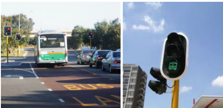
Fig. 3.5 Dedicated bus lane and different types of signalisation for giving priority
