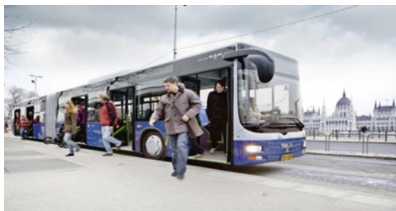
Fig. 2.25 City bus with five wide doors. Presented by MAN in the EBSF project (European bus systems for the future 2011)
