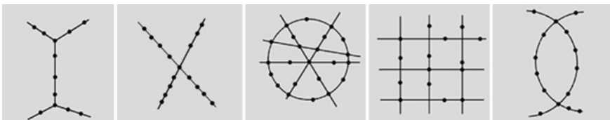
Fig. 2.18 Examples of rail network structures: diametrical with branching (X-system), radial (cross-system), circle-radial system, intermeshed-system and air-bladder system
