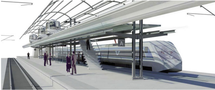
Fig. 8.3 Transfer terminal between train and PRT
