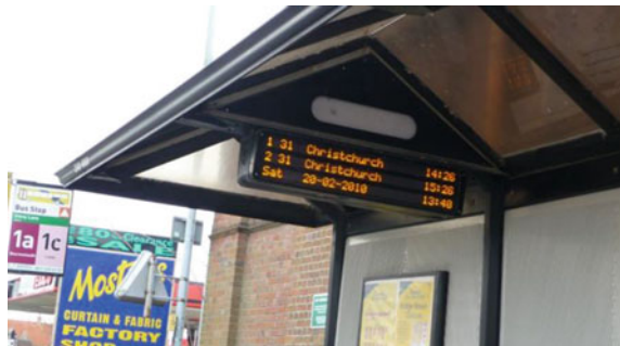
Fig. 3.14 Real-time information panel at a bus stop
