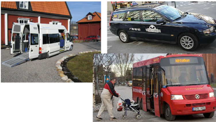
Fig. 2.30 Vehicles used by the STS in Stockholm: low floor minibus, Taxi and Midibus. The latter for bus-on-demand services ( photographs Hans Adeby, SL Stockholm, Public Transport Authority SLL)
