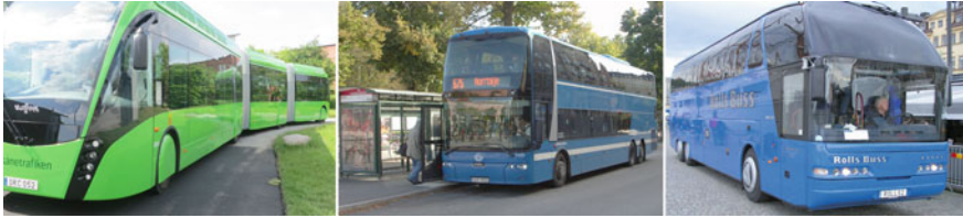
Fig. 2.10 Example of bus types. A double-articulated BHS bus, a regional double-decker and a long-distance tourist coach ( photographs Kottenhoff )
