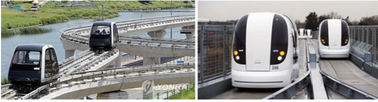
Fig. 2.31 Personal rapid transit systems (Vectus) in Suncheon S Korea and at Heathrow airport (photographs Yonrap News and Kottenhoff)
