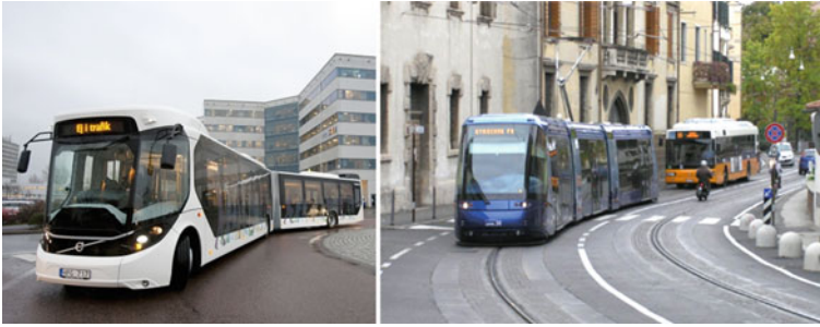
Fig. 2.28 Volvo concept bus for the EBSF project (Volvo Bus) and Translohr rubber wheel tram, “Tram on Tire” in Padua, Italy ( photograph Kottenhoff 2008)
