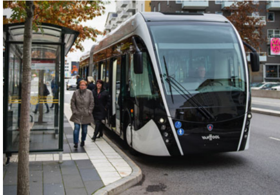
Fig. 2.15 A bulb or heel stop in Stockholm with a prototype VanHool/Scania BHS vehicle (photograph Scania)
