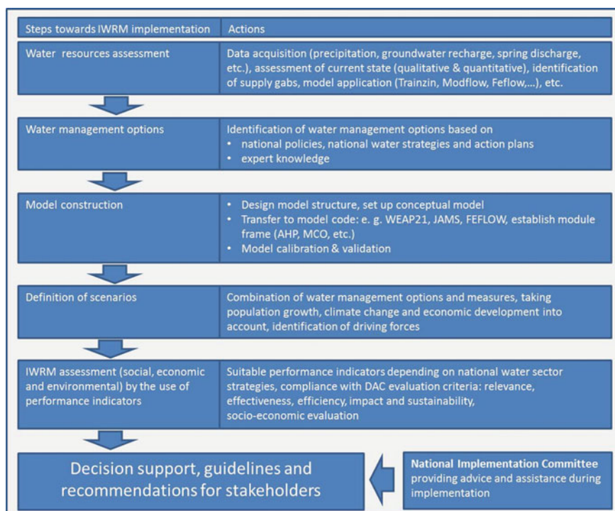
Fig. 28.4 Scheme for the setup of an IWRM approach developed for the Wadi Shueib
