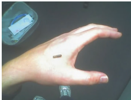
Fig. 5.1 An RFID sensor implanted in the hand. The microchip contains stored information which can be transmitted to a reader and then to a computer. RFID’s can be passive, semi-passive or active. Active RFID’s have an internal power source such as a battery, this allows the tag to send signals back to the reader. Image from Amal Graffstra, Wikipedia Commons
