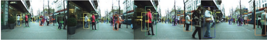
Fig. 6.1 The tracking system developed by University of Washington researchers first systematically picks out people in a camera frame, then follows each person based on his or her clothing texture, color and body movement. Image courtesy of Professor Jeng-Neng Hwang, University of Washington
