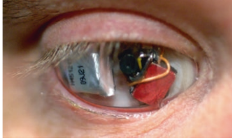
Fig. 2.2 The Eyeborg Project began when one-eyed filmmaker, Rob Spence decided he wanted a prosthetic eye with a video camera in it. The device contains a miniature camera and micro RF transmitter that can send out what Rob's eyecam sees to a receiver and beyond. (Image Courtesy of Rob Spence)
