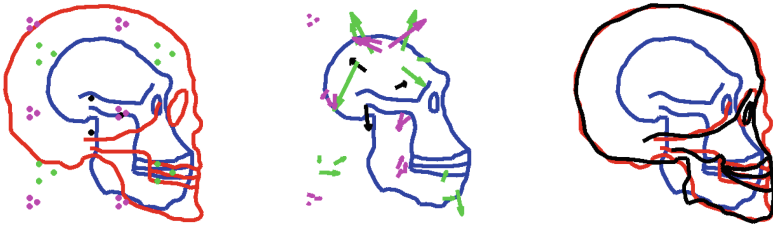
Fig. 7. Matching from f_0 (blue) to f_1 (red), with parameters per scale ( \sigma_1 : black, \sigma_2 : green, \sigma_3 : magenta). Left: initialization geometrical descriptors. Middle: Optimized initial geometrical descriptors and controls. Right: Match at t = 1 (black) (Color figure online).
