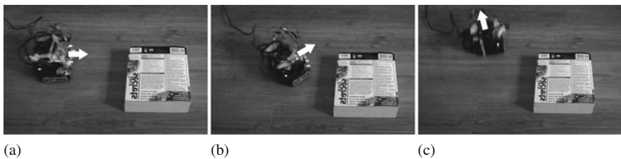
Fig. 4 Three frames taken from a video of the obstacle avoidance experiment. a The robot moving forward detects an object b the robot turns towards the closest unobstructed path, c once the path ahead is clear the robot continues to move forwards
