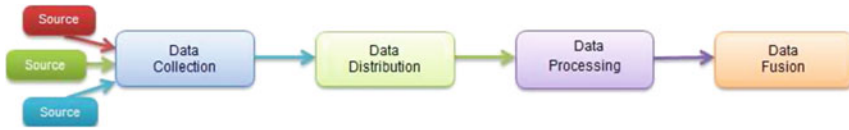
Fig. 1 Main functional blocks of a real-time intelligent event correlation system
