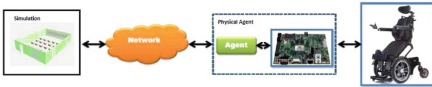
Fig. 6 Connection between the real robot and the virtual one
