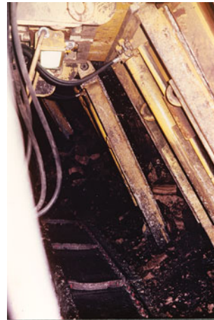
Fig. 9.31 A Hemscheidt LTCC face with gates incorporated into the shield plates, operating at Velenje, Slovenia (After Galvin 1978)
