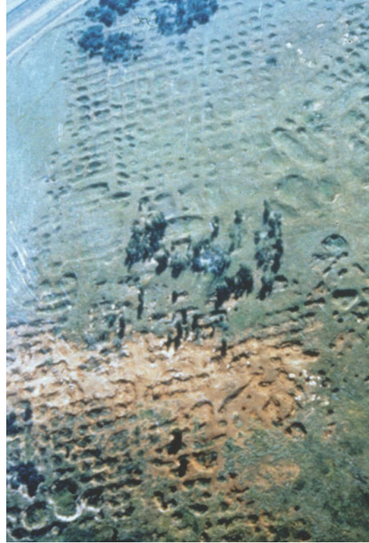
Fig. 3.35 Surface expression of a mixture of intersection falls and bord collapses over bord and pillar workings at shallow depth
