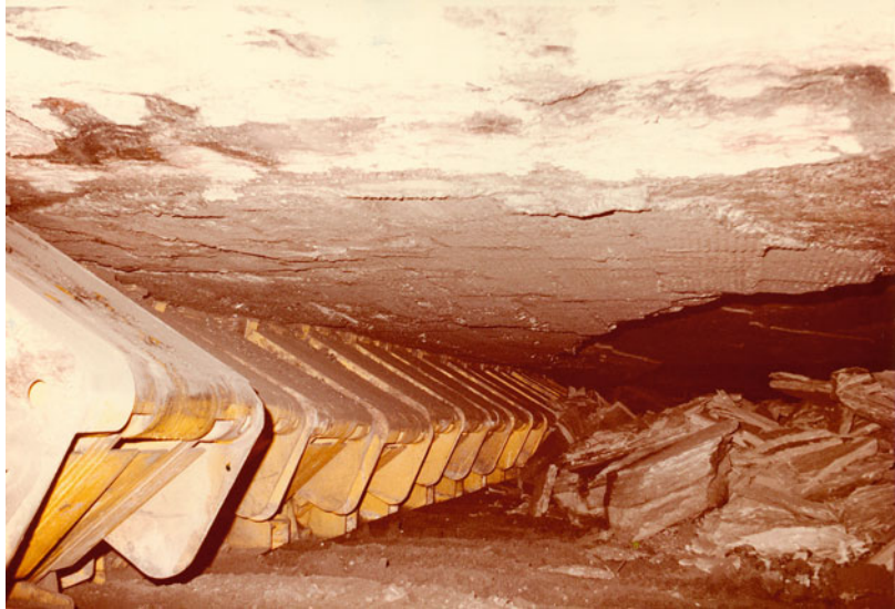
Fig. 3.20 Caving behaviour of moderately strong, bedded roof strata at the gate-end of a longwall panel during the early stages of retreat
