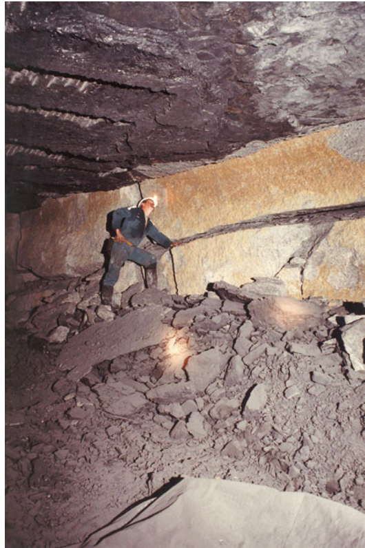
Fig. 8.25 A goaf fall along a pre-existing open joint plane or ‘water crack’
