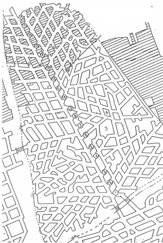
Fig. 4.9 An example of irregular bord and pillar workings (After Anderson 1993)
