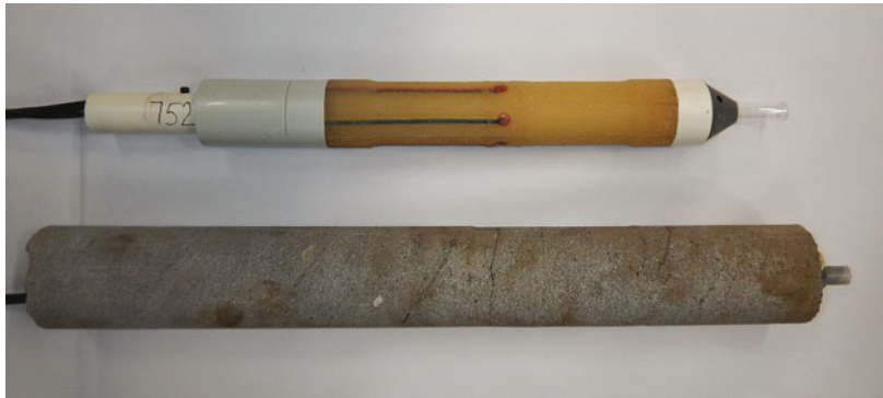
Fig. 12.15 An ANZI borehole stress measurement cell in both an uninstalled state and embedded in an overcore
