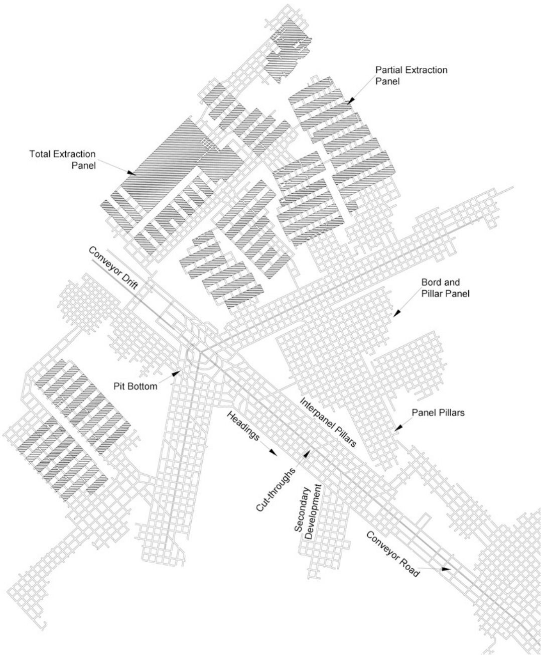
Fig. 2.2 Mining terminology illustrated with the aid of a mine layout designed for bord and pillar mining and selective secondary pillar extraction
