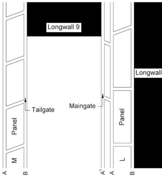
Fig. 5.6 The concept of a 'sacrificial gateroad' as employed in a high horizontal stress environment at Appin Colliery, Australia, to create a stress shadow in which to subsequently drive the maingate (Modified from Todd 1983)
