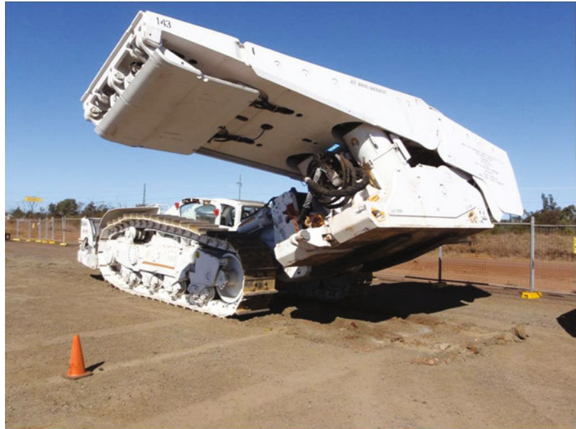
Fig. 9.15 A 2 leg, 17.5 MN capacity, shield powered support fitted with an articulated flipper
