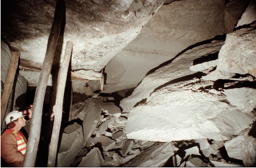
Fig. 3.8 Caving of a moderately strong massive roof, illustrating attributes of a flat caving angle and a high initial bulking factor
