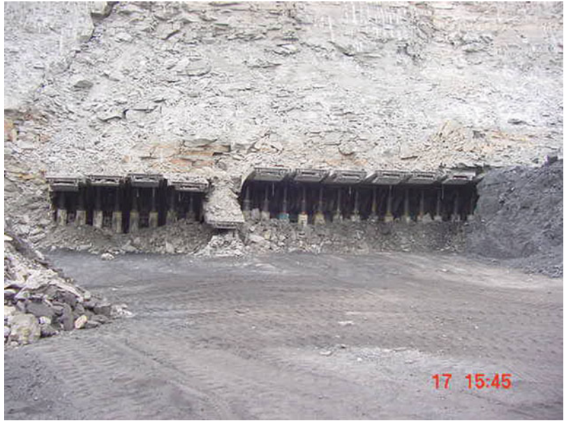
Fig. 3.12 Exposed goaf showing angle of break at the side abutment of a shallow, supercritical width, longwall panel in a weak immediate roof strata environment at a depth of approximately 70 m
