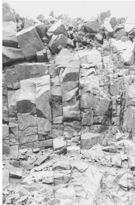
Fig. 3.22 An example of the structural fabric of a dolerite sill after it has been impacted by blasting in a quarry (After Galvin 1982)
