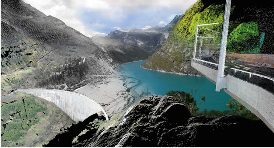
Fig. 1 Generated data visualization image. Combination of pointcloud data from airborne and terrestrial laser scan. Image by Pascal Werner
