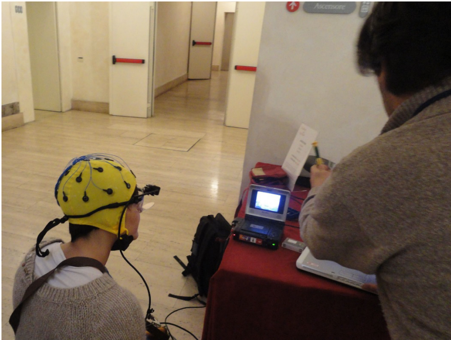
Fig. 2. The typical setup for the recordings employing the international 10–20 system for the electrode montage and the ASL eyetracker device. The mobile EEG and eyetracker devices was worn by the subjects without any relevant physical efforts.
