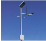
Fig. 1. A REDE WSN node deployed in São Carlos - SP, Brazil.
