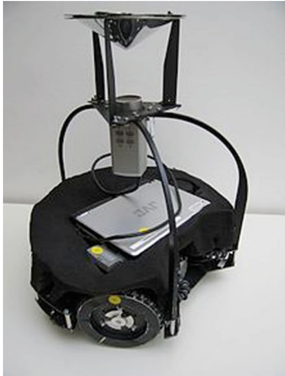
Fig. 2.3 A wheeled robot with an omnidirectional camera. (This image is in the public domain and was downloaded from Wikipedia, Omnidirectional camera)
