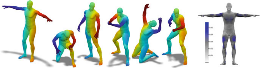
Fig. 10.3 Dense point-to-point correspondences obtained between the left TOSCA human shape and its approximate isometries. Corresponding points are marked with consistent colors. The average correspondence distortion is depicted in units of the reference shape diameter. The highest distortions are obtained on the non-isometric joints, but do not exceed 6 % of the diameter
