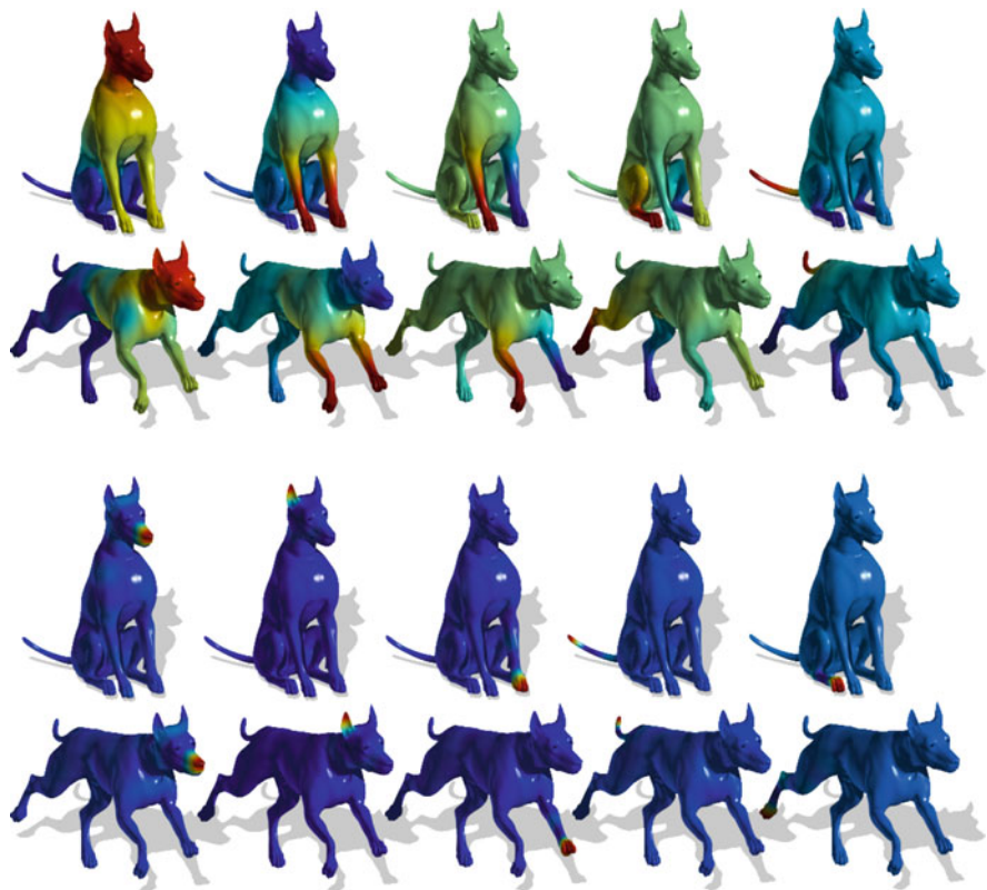
Fig. 13.6 Mapping functions between two almost isometric shapes via our spectral matching. Top : eigenfunctions of the Laplace-Beltrami operator. Bottom : smoothed point indicator functions
