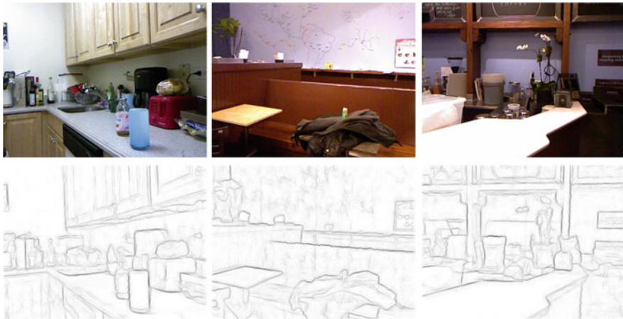
Fig. 7.3 RGB-D boundary probabilities produced by Dollár and Zitnick [8] on examples from NYU Depth (v2)
