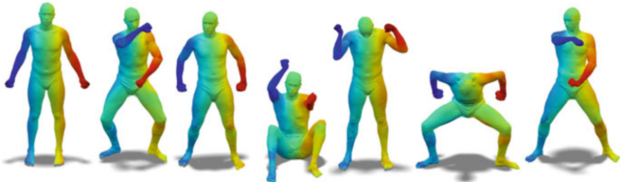
Fig. 10.4 Dense point-to-point correspondences obtained between the left SCAPE human shape and various other poses. Corresponding points are marked with consistent colors
