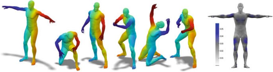
Fig. 10.3 Dense point-to-point correspondences obtained between the left TOSCA human shape and its approximate isometries. Corresponding points are marked with consistent colors. The average correspondence distortion is depicted in units of the reference shape diameter. The highest distortions are obtained on the non-isometric joints, but do not exceed 6% of the diameter
