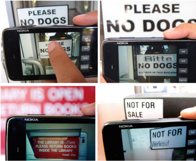
Fig. 1.1 Top row TranslatAR in operation. The user detects the text he or she wishes to translate and taps on it ( top left ). The system automatically detects the extent of the text, extracts the letters via OCR, and produces a translation, which is then presented as a live augmented reality (AR) overlay ( top right ). Bottom row TranslatAR used in two other situations
