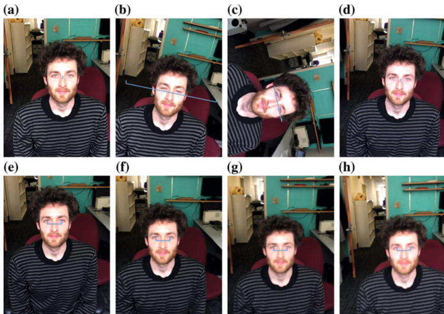
Fig. 14.15 The white ruler in each frame shows our algorithm’s estimation of inter-pupillary distance given the data up to that point in time. The estimation converges once the phone undergoes translation after 3 s. True pupil distance is 64.0 mm; final estimated pupil distance is 64.1 mm (0.16 % error). a 0.0s, 0.0 mm. b 1.0s, 421.9 mm. c 2.0s, 154.3 mm. d 3.0s, -0.0 mm. e 4.0s, 66.0 mm. f 5.0s, 63.1 mm. g 6.0s, 62.8 mm. h 7.0s, 64.1 mm
