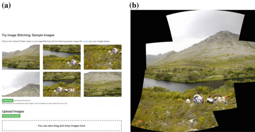
Fig. 11.16 Image stitching web interface. a Sample images and upload interface. b Result for the sample images
