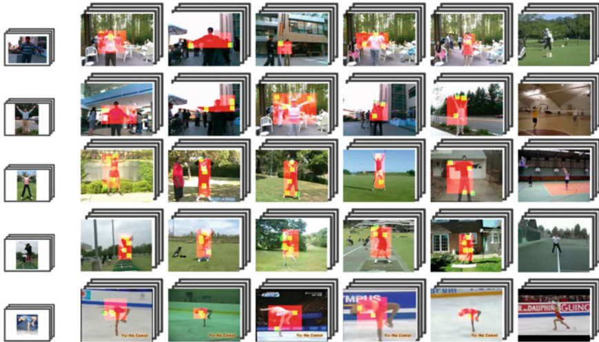
Fig. 13.4 Sample results of thematic action discovery. From top to bottom , the actions are Hand Clap, Hand Wave, Jumping Jack, Golf Swing, and Figure Skating Spin, respectively. The discovered thematic actions are located by the red bounding boxes , and the videos without bounding boxes contain non thematic actions. The cohesive STIP features are also shown, and most of them are inside the bounding box
