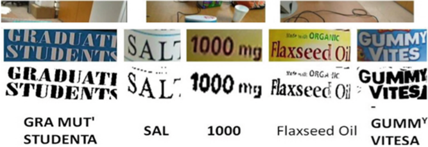
Fig. 9.12 a Some results of text detection on the blind user-captured dataset, where localized text regions are marked in blue. b Two groups of enlarged text regions, binarized text regions, and word recognition results from top to bottom [10]
