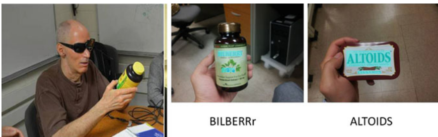
Fig. 9.11 Prototype system assists blind user read text information from handheld objects, including the detected text strings in cyan and the recognized text codes
