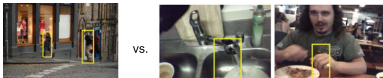
Fig. 4.2 Understandably, while effective for human-taken photos ( left ), today’s best object detectors break down when applied to egocentric video data ( right ). Each image displays the person detections by the DPM [9] object detector
