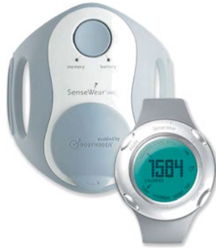
Fig. 8.4 SenseWear Armband Pro 3 activity monitor; it uses acceleration, skin temperature, heat flux, and galvanic skin response to estimate energy expenditure (kcal/day). (© Image courtesy of BodyMedia, Inc.)
