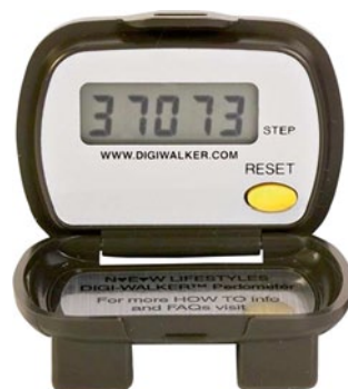
Fig. 8.1 Yamax SW-200 spring-levered pedometer. (Figure courtesy of Dr. Teresa Vollenweider)
