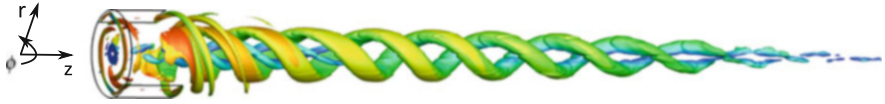
Fig. 6 Helical vortex in the swirl tube for the swirl number S = 5.3 and Re = 10,000 , iso-surfaces of Q = 1 , color = axial velocity [5]
