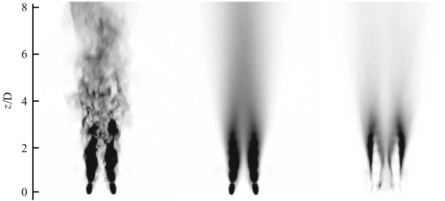
Fig. 2 Snapshot ( left ), temporal averaged ( middle ), and fluctuations ( right ) contours for axial velocity (levels from 0 to 700 \text{ m s}^{-1} for the velocity and 0 \text{ m}^2 \text{ s}^{-2} to 3 \times 10^5 \text{ m}^2 \text{ s}^{-2} for the fluctuations; color scales from white to black )
