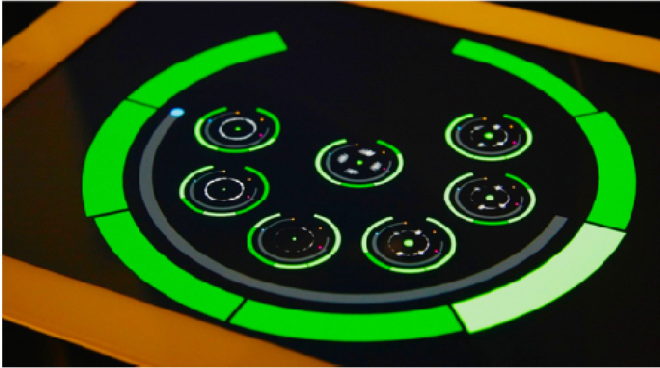
Fig. 1. The c3n play app version 1.0 running on an iPad 3 device. The photograph shows a zoomed in view of an arrangement of audio loops called a performance. Each performance consists of seven scenes indicated by the green circle segments around the performance. Each loop can be attached to any of the seven scenes. The current playing scene indicated by a fully saturated green colour.
