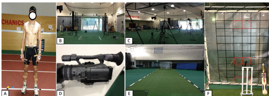
Fig. 1. (A) Bowler with 48 markers at key anatomical landmarks. (B, C) Motion capture volume and camera set up at AIS. (D) Sony Handicam HDR FX7 mounted above the bowler's head to estimate the delivery types. (E) View of the artificial turf (F) The calibrated area with distinct red squares for targeting aim.
