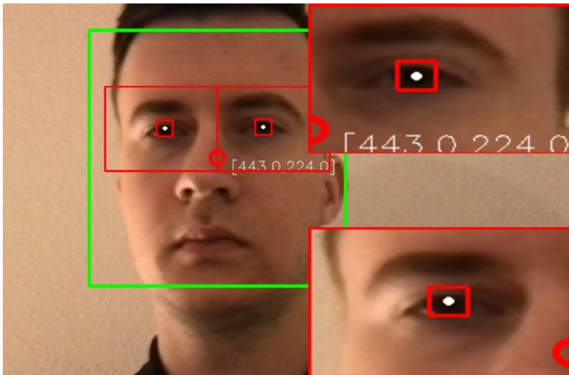
Fig. 5. Example of finding faces and eyes using OpenCV library
