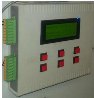
(d) A gateway transmitting measurements from the electric meter in Fig. 1c
