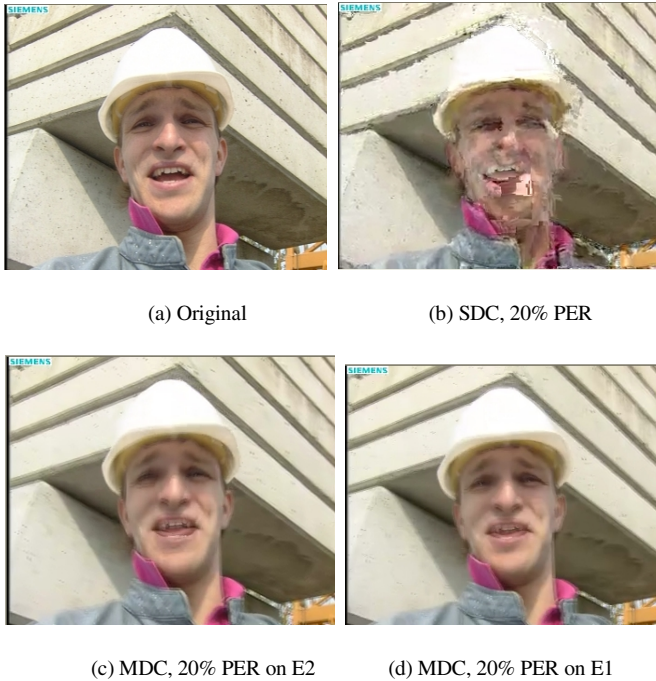
Fig. 4. Subjective quality of video transmission in ideal MDC channel for underlay CR.
