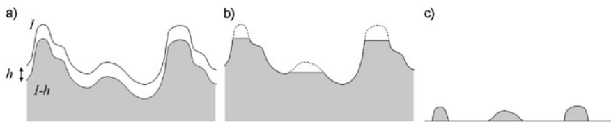
Fig. 4 The H-maxima transform extracts peaks higher than h . (a) Original image I , subtracted by a scalar h . (b) Greyscale reconstruction of I using I-h as marker. (c) Subtraction of grey scale reconstruction from original image
