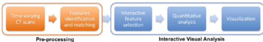
Fig. 2 The workflow of the proposed approach. In the pre-processing stage, features in a dynamic CT data set are extracted and matched between scans. In the second stage, user can interactively select FOIs. Based on the information from the pre-processing stage, selected FOIs are tracked automatically in the time domain. Depending on the application in mind, different quantitative measurements can be performed and visualized for assessment
