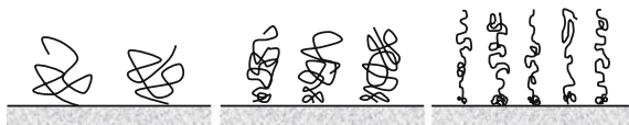
Fig. 1.13 As the grafting density of polymer chains at an interface increases from left to right we observe a ‘mushroom’, ‘overlapping mushroom’, and finally at high densities a ‘brush’ regime
