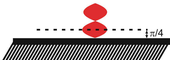
Fig. 14.7 Standing wave pattern formed by a reflected electromagnetic wave that is impinging on a metal surface at normal incidence. The pattern formed by interference between incident and reflected wave has a knot at or near the surface. The maximum of intensity is somewhere around a quarter of the wavelength inside the incidence medium
