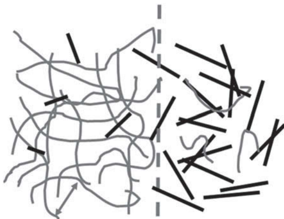
Fig. 6.1 Schematic impression of a water–water interface, formed by the phase separation of two aqueous solutions containing two different polymers. The interface is permeable for water, salt and the low molar mass fraction of the polydisperse polymers
