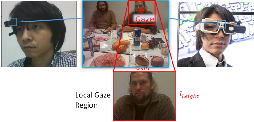
Fig. 1. Wearable eye trackers. Left) PupilLabs Eyetracker, Right) SMI ETG with Brother AirScouter (HMD), Middle) Scene camera image, and Bottom) Cropped local gaze region.
