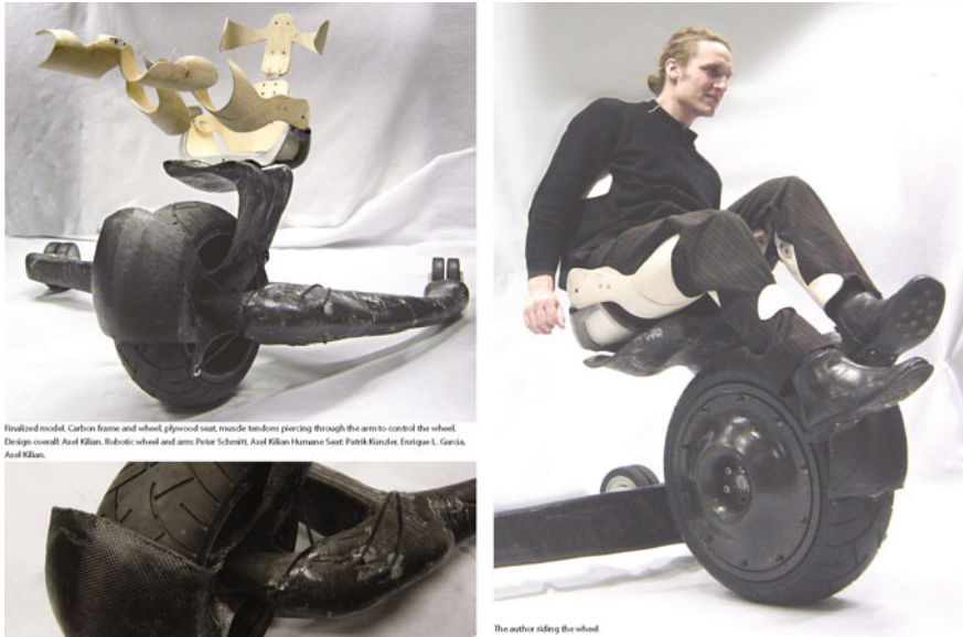
Fig. 9 Final selective prototype in carbon fiber, Axel Kilian, Peter Schmitt, Patrik Künzler, Enrique Garcia (Kilian 2006a)
