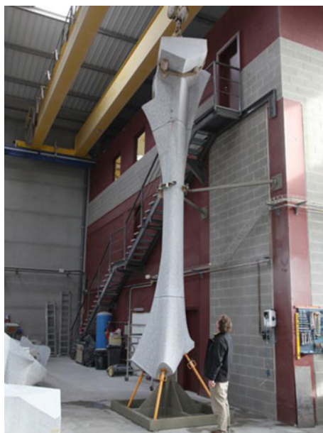
Fig. 23 Final nine metre high column at the site of its NC cutting
