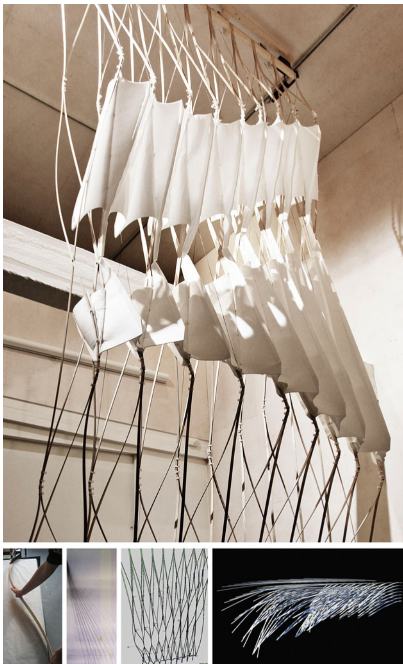
Fig. 2 Thicket and Thaw: material prototypes are used to inform digital design models of the formal properties of material deformation. Digital prototypes are used to simulate aggregate behaviour of structural assembly
