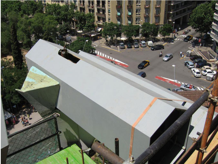
Fig. 20 Full-scale prototypes that could be moved backwards and forwards to gauge the optimum overhang
