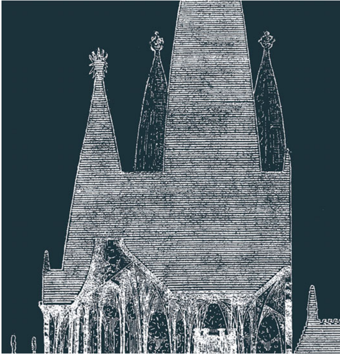
Fig. 4 Close-up of the section with the hatched-out enclosed space above the crossing (Sala Creuer)
