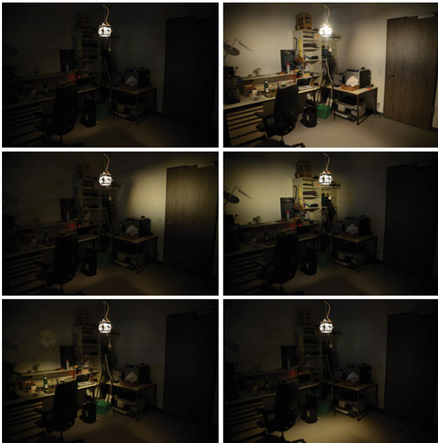
Fig. 23 Users can control the individual faces of the lamp to create desired lighting situations
