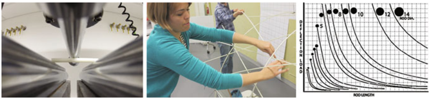
Fig. 8 Bending testing and prototyping connections with varying thicknesses of GFRP rods
