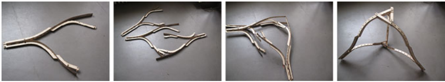
Fig. 4 Dermoid: physical prototypes ideation detailing of a double layered system of zipped flanges and webs. All connections are friction only
