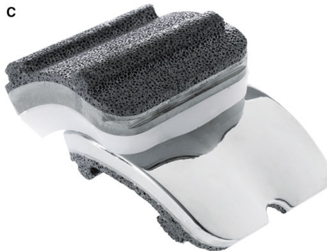
Fig. 12.2 Implant design. Medially, the talar articular surface has a smaller radius of curvature (a, b), allowing continuity during ankle joint range of motion and mimicking the frustum of a cone (c). Images utilized with permission from Zimmer
