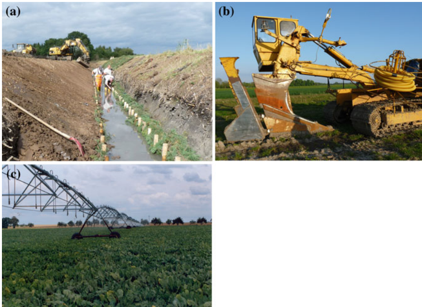
Fig. 10 Examples of modern drainage and irrigation technology: a Well-constructed ditch for land drainage and water table control, b Laser-controlled machine for trenchless subsurface drainage, c Automatically operating low-pressure sprinkler irrigation machine. It is likely that these and further technology and knowledge about their operation will be needed to exploit the higher land use potential of a warming Siberia. Their application requires complex planning, careful construction, operation and maintenance to achieve their main effects and to minimise negative side effects
