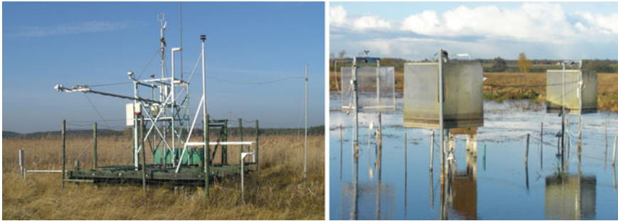
Fig. 4 Automatically operating eddy-flux and chamber measurement stations for analysing and modelling the carbon balance on different kinds of peatlands. Left eddy-flux station developed by the Meteorology Department of the Poznan University of Life Sciences, Poland. Right chamber measurement station operated by ZALF Müncheberg, Germany. Peatlands created in temporal ponding phases are characterised by particularly high methane emissions
