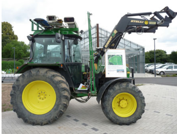
Fig. 9 Methods of precision agriculture can help to optimize fertiliser demands according to the spatio-temporal specific conditions of crops. The photo shows an “N-sensor” mounted on a tractor. It is combined with a GPS system and can be a basis for the operational control of fertiliser application
