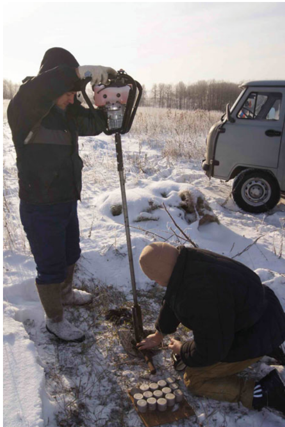
Fig. 2 Soil sampling for water content. Another measurement has to be carried out in spring before, during, and after the snowmelt. Volumetric samples from core cylinders are important to calculate the amount of water which infiltrates the soil during the snowmelt
