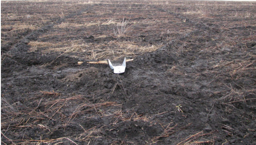
Fig. 1 Short-term runoff plot with a minimum size of 30 \times 5 m
