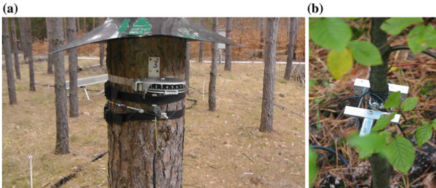
Fig. 9 a Dendrometer measuring the radial increment on a pine tree (manual reading and continuously measuring). b Continuous measurement on a small beech tree
