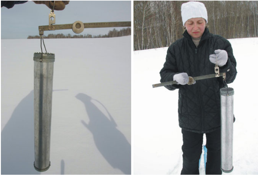
Fig. 5 Calculating the snow water equivalent. The mechanical balance is a very robust and reliable solution under severely frosty conditions
