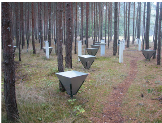
Fig. 8 Measuring field with litter fall samplers in a pure pine stand
