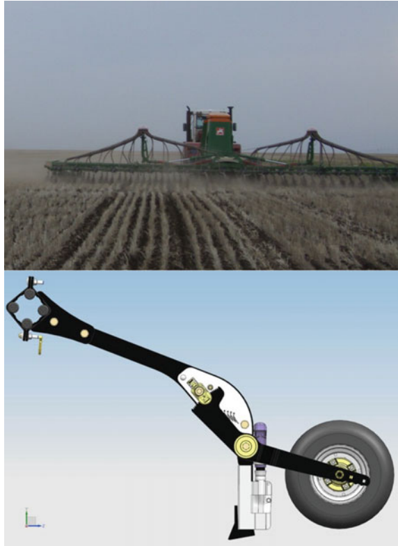
Fig. 13 No-Till—Airseeder CONDOR 15001-C Wind-stopper effect due to standing stubble after seeding with single guided narrow hoe opener systems (author’s photos 2009/2012, shank scheme courtesy of Amazone company, Germany)
