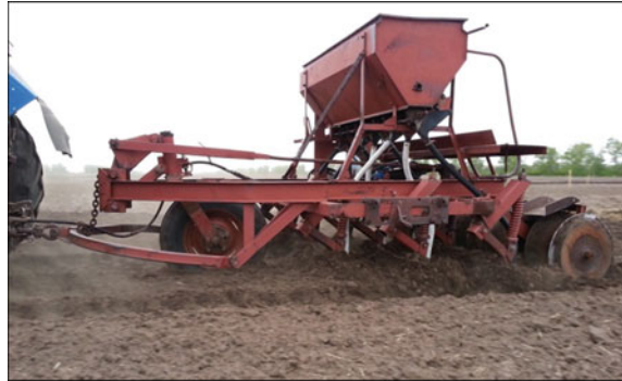
Fig. 15 Mechanical chisel opener drill C3C 2.1, no single guided shanks, heavy soil disturbance while opening the furrow
