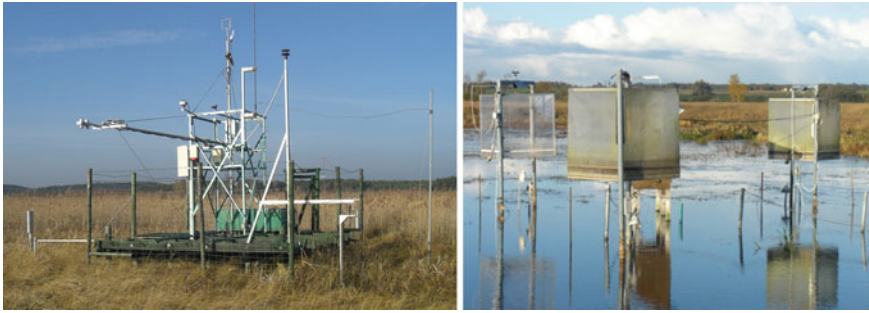
Fig. 4 Automatically operating eddy-flux and chamber measurement stations for analysing and modelling the carbon balance on different kinds of peatlands. Left eddy-flux station developed by the Meteorology Department of the Poznan University of Life Sciences, Poland. Right chamber measurement station operated by ZALF Müncheberg, Germany. Peatlands created in temporal ponding phases are characterised by particularly high methane emissions
