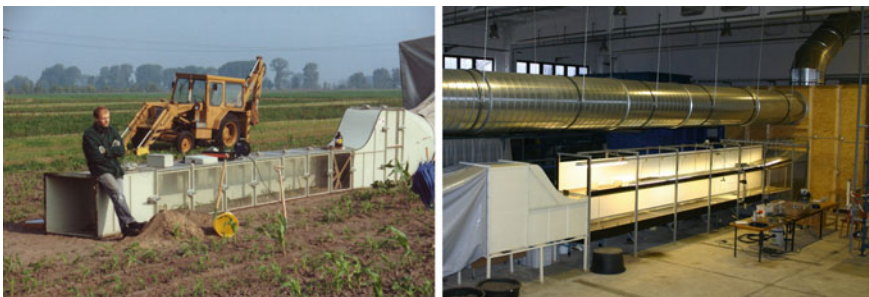
Fig. 10 Mobile and stationary wind tunnel used by the author
