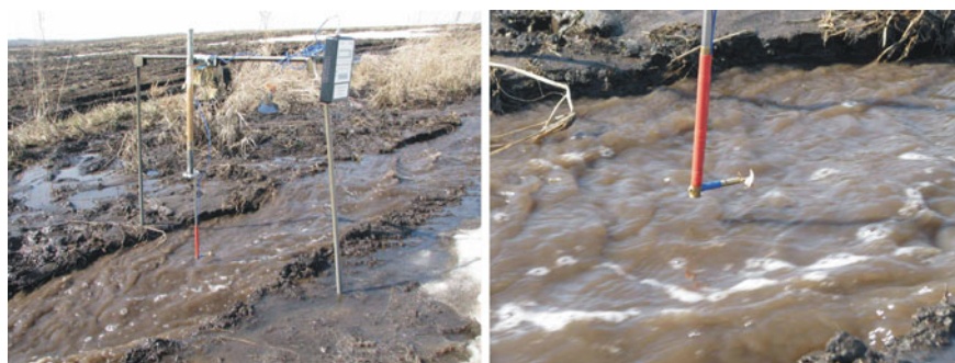
Fig. 6 Determining the speed of a water stream using a “GR-99” hydrological rotator
