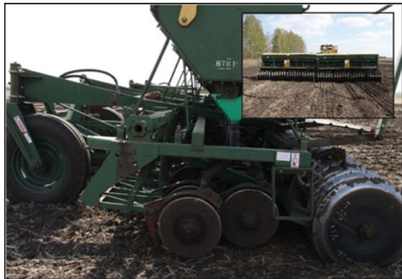
Fig. 14 Mechanical drill C3Π 3.6—double disc opener only just cuts through straw, for use after seedbed preparation only
