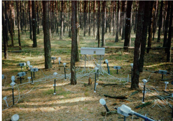
Fig. 6 Measuring soil moisture and water retention in a Scots pine forest
