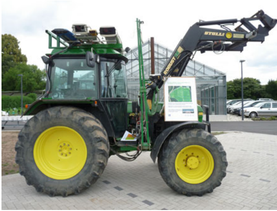
Fig. 9 Methods of precision agriculture can help to optimize fertiliser demands according to the spatio-temporal specific conditions of crops. The photo shows an “N-sensor” mounted on a tractor. It is combined with a GPS system and can be a basis for the operational control of fertiliser application
