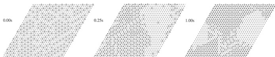
Fig. 5.49 Series of snapshots after a negative-going potential step to 20 mV below the transition between the low coverage and mixed layers, see arrow A in Fig. 5.46a. Note the high concentration of sulfate species at 0 s, the predominance of phase (\sqrt{3} \times \sqrt{3})_{1/3}^{1/3} at 0.25 s and the predominance of the (\sqrt{3} \times \sqrt{3})_{2/3}^{1/3} at 1 s. The circles were drawn to focus on some compact, representative domains (Reprinted with permission from Ref. [94])
