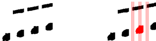
Fig. 8. Linked notes without stems and sets of lines to recognize eighths and sixteenths
