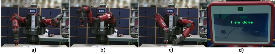
**Fig. 5.** Baxter performing an instance of the GIG shown in Figure 3. First, Baxter picks up the orange block (a); then Baxter checks if a location is unobstructed with its left arm camera (b); Since the location is unoccupied, Baxter drops the Block. (c); Finally, Baxter says that it is done (d).
