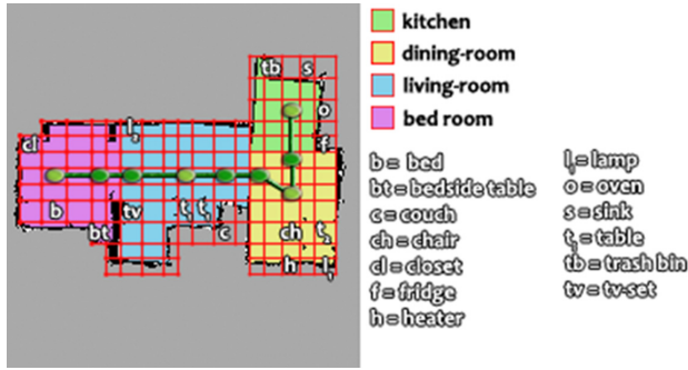
Fig. 3: Semantic map of a domestic environment. The Topological Graph is depicted on top of the Cell Map and the objects in it. The metric map is also depicted in the background.
