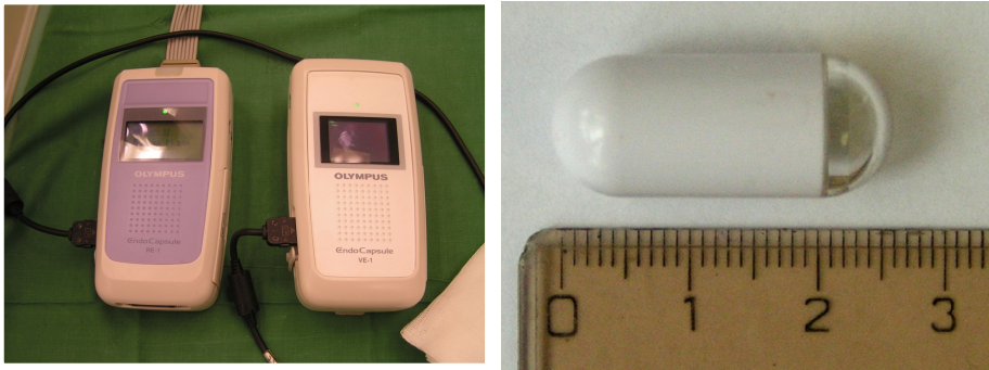
Fig. 1. The wireless capsule endoscope is a disposable capsule with an outer diameter of 11 mm, length of 26 mm and weighing 3.8 g. It moves through the small bowel, propelled by peristalsis and transmits data to a portable data recorder. [3]
