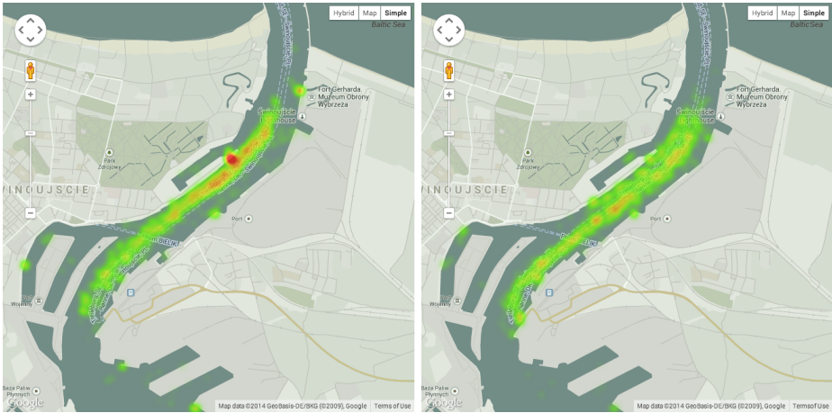
Fig. 4. Traffic patterns for course SW (to the left) and NE (to the right)
