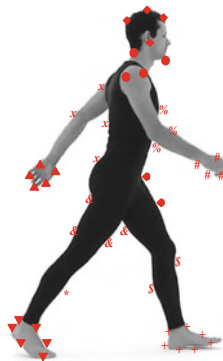
Fig. 6. Image features are segmented into clusters representing independent motions; features with the same symbol belong to the same cluster.
