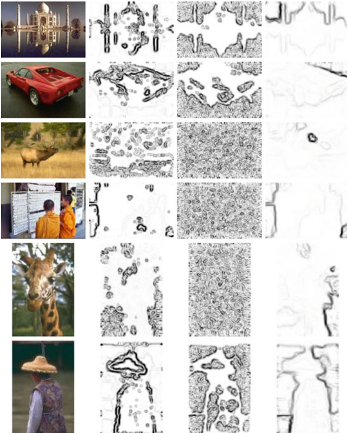
Fig. 6. Edge-detection results with Szemerédi Regularity Lemma + Key Lemma . First column: images from BSDS500. Second column: edges for d = 0.44 and \epsilon = 0.51 . Third column: edges for d = 0.44 and \epsilon = 0.71 . Fourth column: edges from quantum walks for \alpha = 0.1 without compression.
