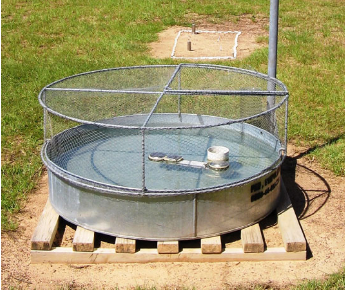
Fig. 4.3 Evaporatory pan used to measure daily evapotranspiration water losses
