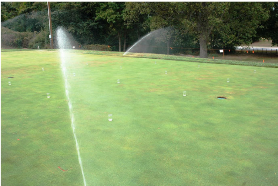
Fig. 4.9 Conducting a distribution uniformity test when calibrating an irrigation system to determine how uniform water is being applied
