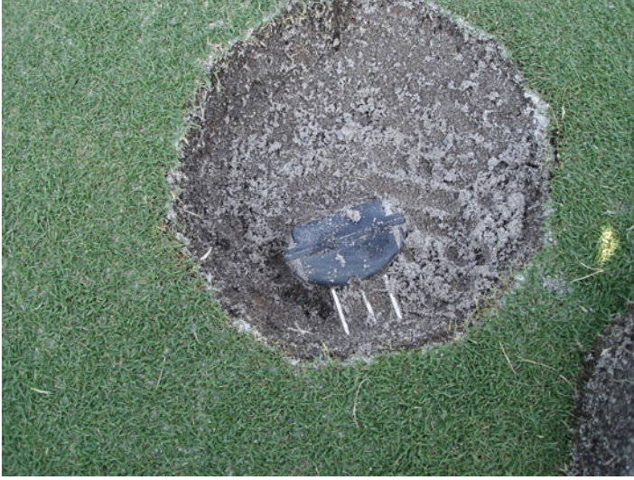
Fig. 4.4 Soil moisture dielectric probe with two sets of probes used to measure quantitative levels of soil moisture near the soil surface and several inches (turfgrass rootzone) below this
