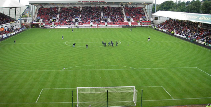
Fig. 2.51 Soccer fields are constructed with little to no surface slopes which may influence sideline shots. In such instances, subsurface drainage becomes more important means to removing excessive soil moisture
