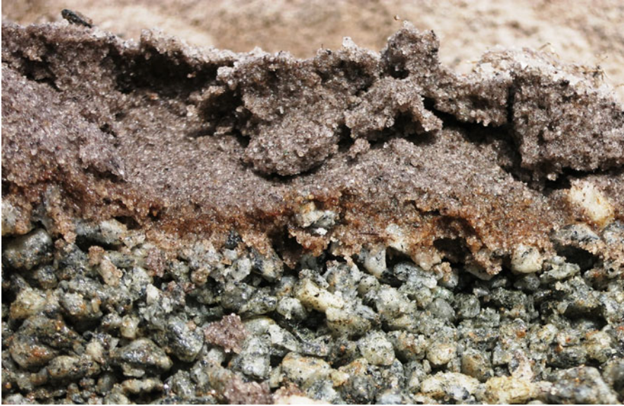
Fig. 3.21 A recent phenomena has been noticed in sand-based rootzone where a layer of orange to rust-colored ferric iron ( \text{Fe}^{+3} ) forms at the interface of the rootzone and underlying gravel drainage bed. This typically originates as a dark gray-colored ferrous iron ( \text{Fe}^{+2} ) at the top of the rootzone and becomes mobile when it encounters anaerobic conditions. Once the ferrous iron contacts the oxygenated gravel layer, it turns into ferric oxide ( \text{Fe}_2\text{O}_3 ) which becomes immobile. The hard, impenetrable ferric iron layer then disrupts normal moisture drainage, causing a higher zone of saturating to develop which may eventually reach the soil surface
