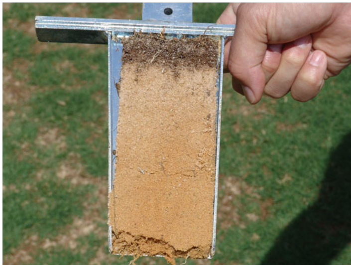
Fig. 2.42 A sand-based sport field rootzone used when fields are built essentially flat. This is necessary to facilitate subsurface drainage since a surface crown is absent
