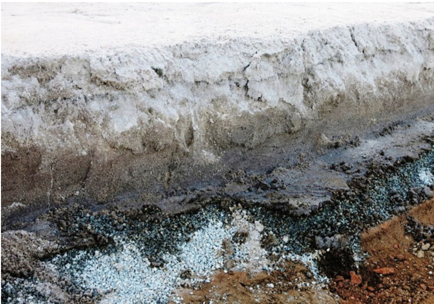
Fig. 3.16 If the gravel's or sand's diameter is too fine in rootzone construction, the zone of saturation may extend into the rootzone, causing drainage and rooting issues
