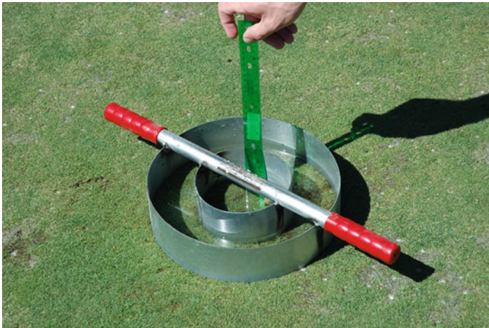
Fig. 1.19 A double-ring infiltrometer being used to measure hydraulic conductivity (internal drainage) of an established turf site
