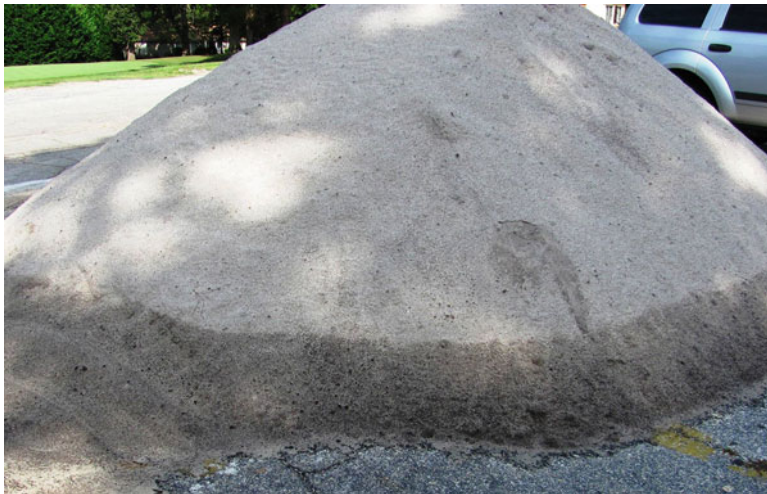
Fig. 1.15 Water height in a sand:peat pile due to capillary action from moisture below. This moisture height is determined by the soil's capillary forces (adhesion and cohesion) against the force of gravity
