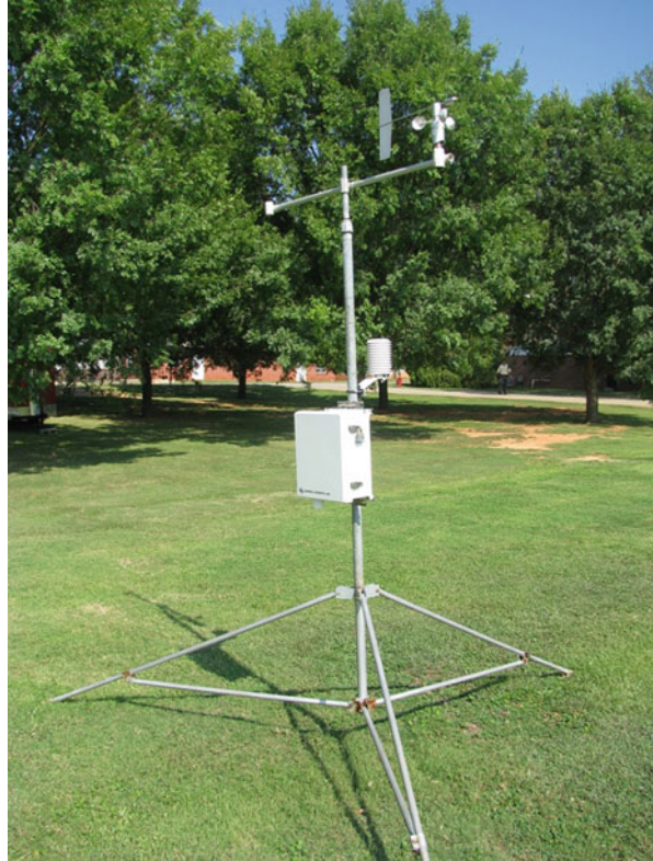
Fig. 4.7 Automatic weather station used to construct predictive models on how much soil moisture is present
