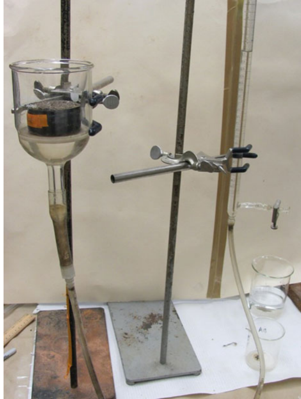
Fig. 1.21 The use of a hanging water column to create soil moisture retention curves for turfgrass soils
