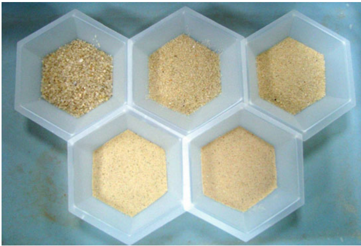
Fig. 3.6 Uniform sands are characterized as having most of the individual particles similar in size, which is termed a narrow particle-size distribution. This is important since like-sized particles do not interpack, and result in good and stable porosity in the soil. By contrast, non-uniform sands have particles ranging from very coarse to very fine in size, and these can interpack and have higher bulk density. Intermediate-sized particles fill the spaces (pores) between the largest particles, smaller particles fill the spaces between the intermediate particles, and silt and clay can fill any remaining spaces. The net result is dense sand with reduced pore space, smaller average pores, and a tendency to compact. Shown are the various sand sizes as defined by the USDA with the coarsest being the upper left and finest lower right
