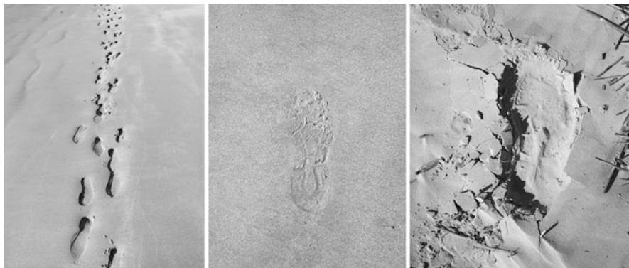
Fig. 1.16 As soil moisture levels change, so do a soil's strength and stability. For example, beach sand, when wet, easily compacts from foot traffic ( left ). As moisture is removed, soil particles become more tightly bonded together and resistance to compression increases ( middle ). As soil moisture is depleted, the soil once again becomes unstable, losing its ability to resist compaction ( right )
