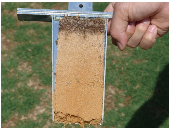
Fig. 3.24 Pure sand fields are not always recommended due to excessive drainage, thus the need for heavy amounts of water and fertilizer, and since most 100 % sand-based fields lack the surface stability and firmness necessary for good footing without excessive tearing of the turf. Pure sand fields also accumulate thatch quicker and more so than fields modified with a small amount of organic matter or native soil
