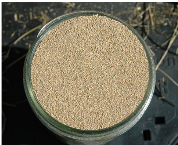
Fig. 3.11 A number of inorganic amendments are marketed as rootzone amendments, and may merit consideration if they are readily available, meet the infiltration and percolation specifications, and are affordable. Shown is a mined highly porous materials that has been processed and sized
