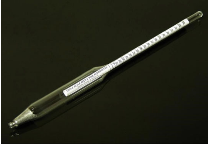
Fig. 1.5 Hydrometer used to separate soil fractions based on its buoyancy in water with soil particles
