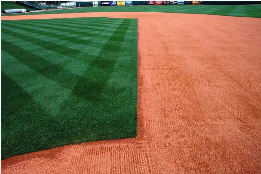
Fig. 2.58 Typical soil of a baseball skinned infield composed of native and calcined clay plus sand
