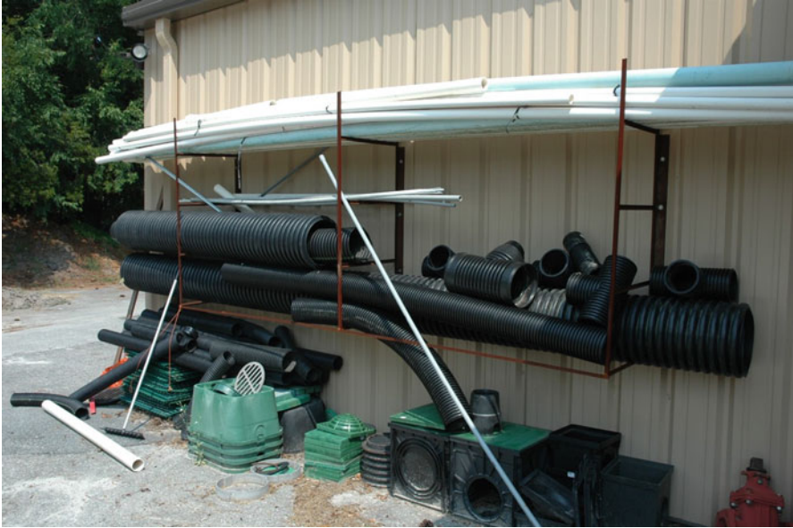
Fig. 2.18 Various sized and types of drainage pipes and other apparatuses used in the turfgrass industry
