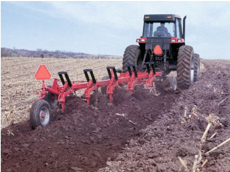
Fig. 1.8 Decreasing soil compaction requires reducing soil mass or increasing soil volume. In traditional agriculture, relieving compaction is often performed by increasing soil volume using various mechanical devices such as plows, harrows, cultivators, roto-tillers, sub-soilers, rippers, etc.
