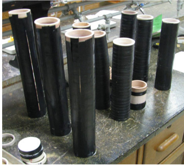
Fig. 1.23 Soil columns used to construct soil moisture retention curves at field capacity
